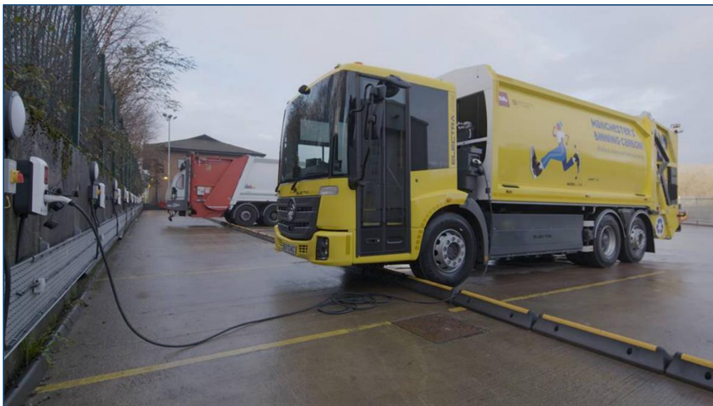
Figure 13-3: One of the City of Manchester's 27 Electra/Mercedes 26 tonne 300 kWh electric refuse vehicles
