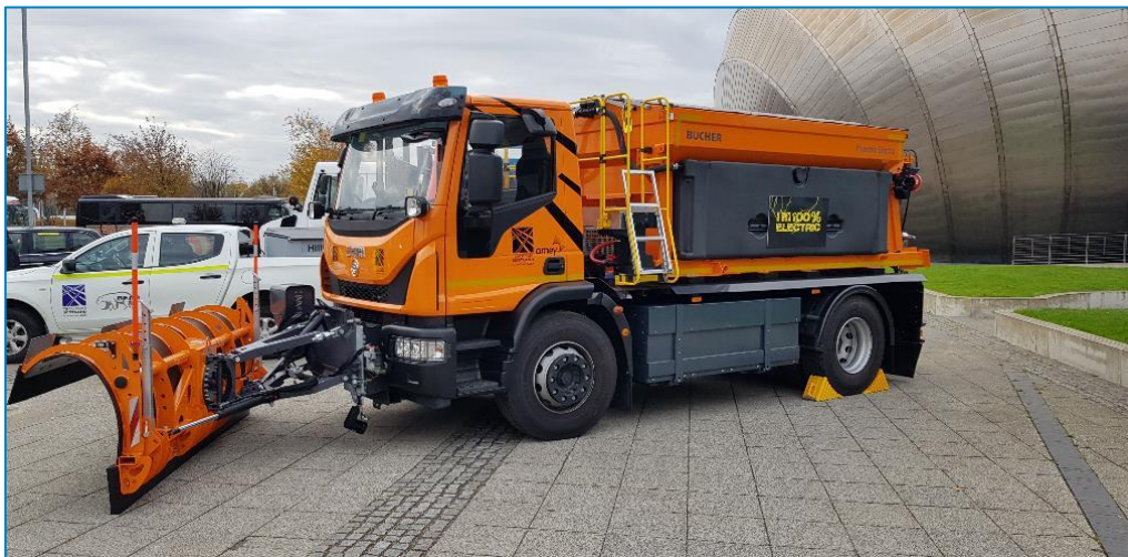
Figure 13-1: Electra Gritter developed for Transport Scotland use on the Forth Bridges
