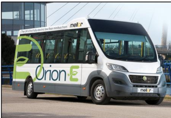
Figure 12-5: Mellor Orion-E 16-seat electric minibus based on Fiat Ducato
