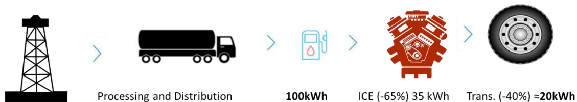
Figure 6-2: Energy efficiency of an internal combustion engine (ICE) vehicle
